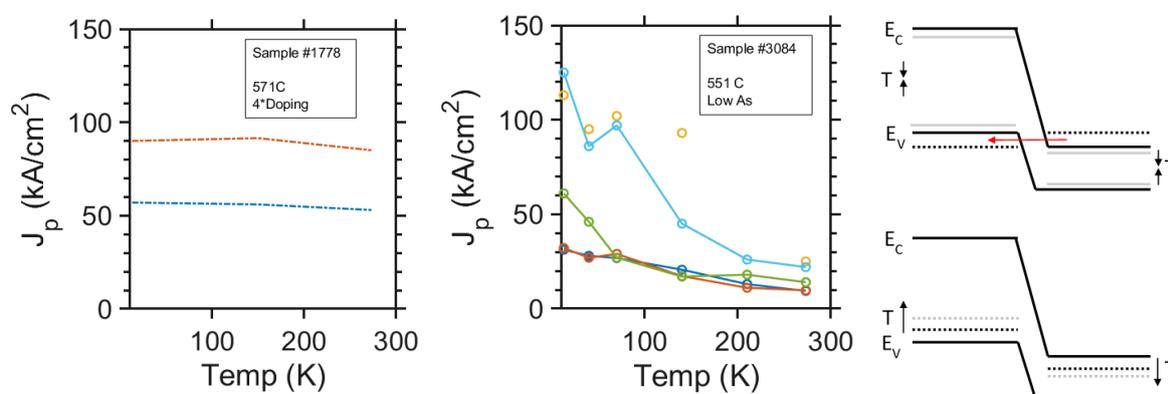
**Fig. 4.5:** Peak current density as a function of temperature for a TFET sample (2 devices) with high (left) and a sample (5 devices) with low source doping (middle, 5 devices). Right: Schematic band structure for a TFET with degenerate doping of source and channel and for a TFET with non-degenerate doping.
