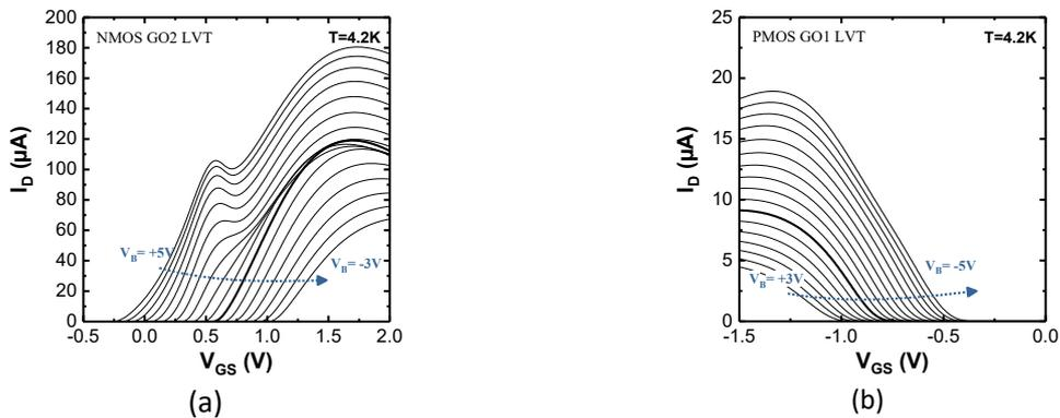
**Fig. 2.11.**  $I_d(V_g)$  characteristics at 4.2K for various  $V_b$  (from -3V to 5V) for a) NMOS GO2 and b) PMOS GO1 devices. PMOS devices do not exhibit the specific feature whatever  $V_b$ .
