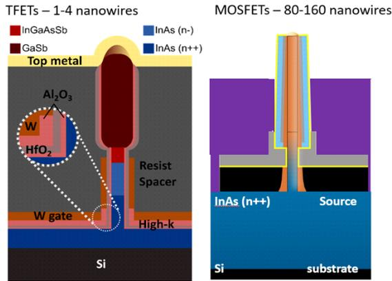
**Fig. 4.1.** Device schematics for InAs/InGaAsSb/GaSb NW TFETs (left) and InAs/InGaAs NW MOSFETs (right).
