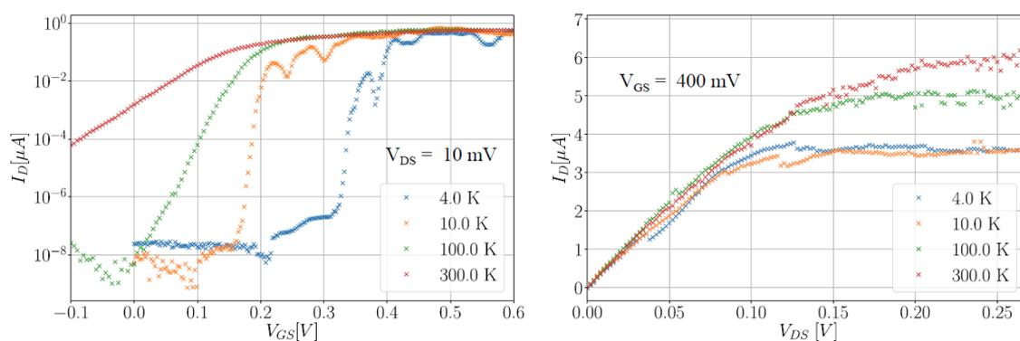
**Fig. 3.3.** Transfer and output characteristics of a FinFET with a single 25 nm wide fin.
