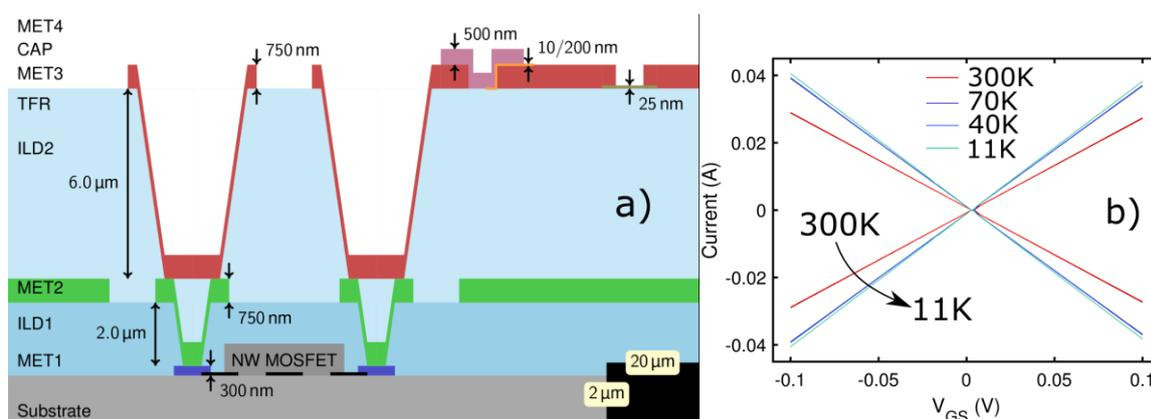
**Fig. 4.6:** (a) A schematic cross-section of III-V compatible BEOL with noted metal (MET<sub>x</sub>), interlayer dielectric (ILD<sub>x</sub>), thin-film resistor (TFR) and capacitor dielectric (CAP) layer, as well as individual height of each of the layers. Via stack is shown as part of device connection. (b) Current-voltage measurements of a via array showing via resistance at room temperature (~300K), 70K, 40K and 11K.
