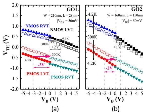
**Fig. 2.6.** Measurements of  $V_{TH}$  vs.  $V_B$  for N- and P-type, RVT and LVT, GO1 (a) and GO2 (b) MOSFETs, at  $300\text{K}$  and  $4.2\text{K}$ ,  $V_{DS} = 50\text{mV}$ .
