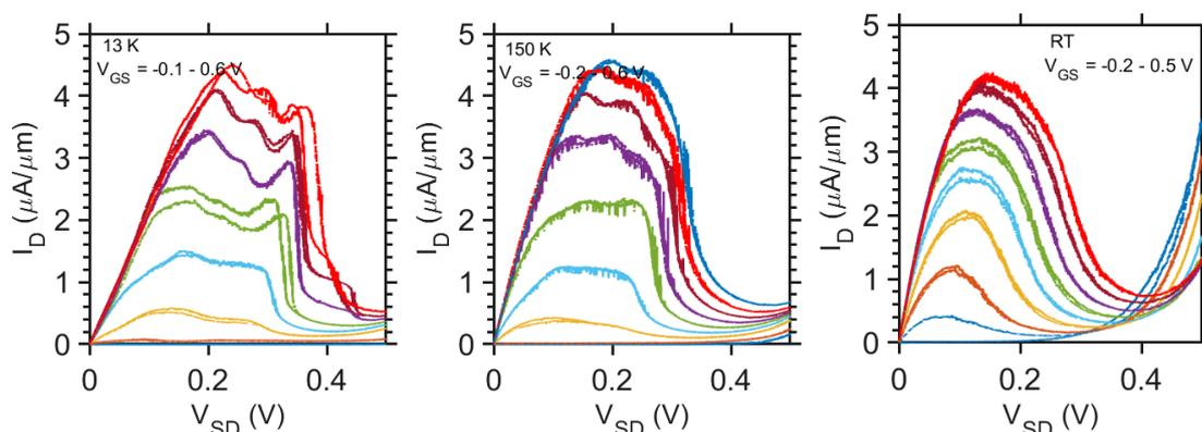
**Fig. 4.4:** NDR characteristics of a vertical nanowire TFET device with higher doping at different temperatures.
