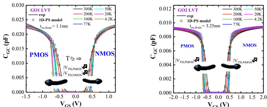
**Fig. 2.2.**  $C_{GC}(V_{GS})$  characteristics for N- and PMOS GO1 and GO2 devices from 300K down to 4.2K, at  $V_B = 0V$ . (Frequency = 1 MHz, AC level = 40mV,  $W = L = 10\mu m$ ).
