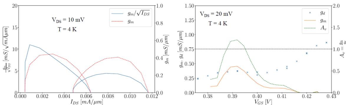
**Fig. 3.6.** Left-hand figure shows the  $g_m/\sqrt{I_{DS}}$  figure of merit, while the right-hand side shows the voltage gain of the measured device above.
