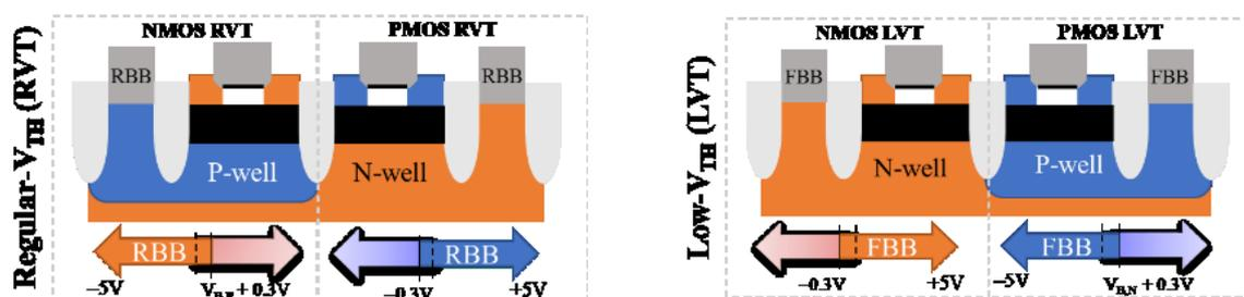
Fig. 2.1. Schematics of 28nm FDSOI N- and PMOSFETs with regular- $V_{TH}$  (RVT) and low- $V_{TH}$  (LVT) flavors.
