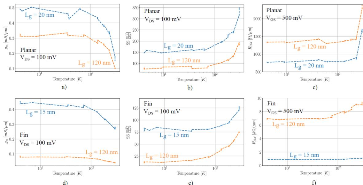
**Fig. 3.2.** Measurement data of planar MOSHEMTs (a)-(c) and lateral InGaAs FinFETs (d)-(f). All three metrics, transconductance, subthreshold swing and on-resistance are measured at 100 mV drive bias.
