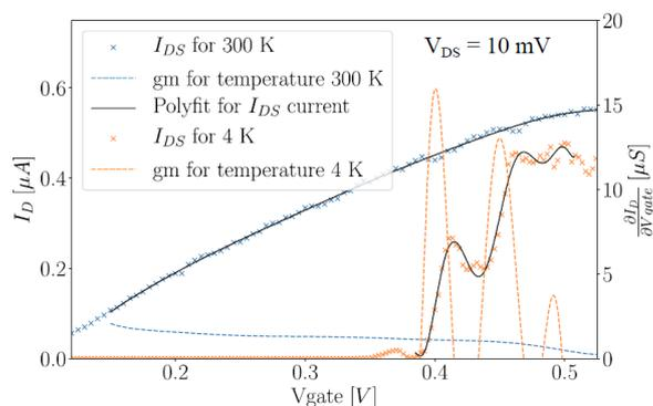
**Fig. 3.4.** Study of the transconductance in a single-fin FinFET. Same device as in Fig. 3.3.
