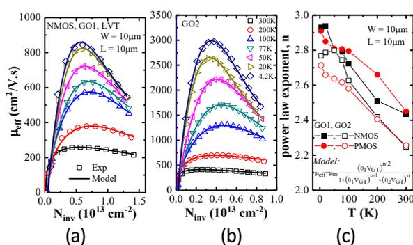
**Fig.2.8.** Experiments and analytical model of  $\mu_{eff}$  vs.  $N_{inv}$  for NMOS GO1 (a) and GO2 (b), varying  $T$ . Power law exponent (c) vs.  $T$  for N and PMOS.
