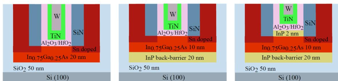
**Fig. 3.1.** Schematic figures of the different device structures that were measured. Left shows a standard InGaAs MOSFET with 20 nm thick channel on BOX. In the middle design the channel thickness is reduced to 10 nm and a 20 nm InP back-barrier is added to protect the back-interface. The right-hand side schematic shows a MOSHEMT design with both top and bottom InP barriers and a 10 nm InGaAs quantum well.
