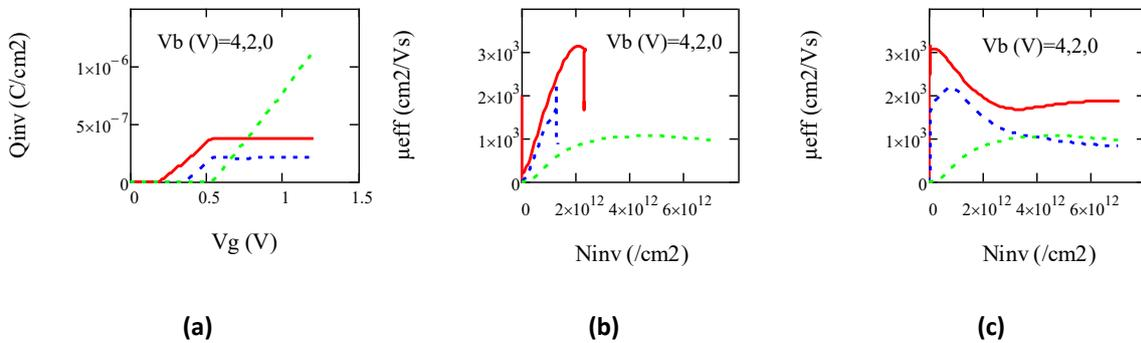
**Fig. 2.10.** a)  $Q_{inv}$  vs  $V_g$  for back channel for  $V_b=2, 4$  V. Green curve shows  $Q_{inv}(V_g)$  for front channel at  $V_b=0$ . b) Back channel  $\mu_{eff}$  vs back channel  $N_{inv}$  and c) back channel  $\mu_{eff}$  vs front channel  $N_{inv}$  for  $V_b=2, 4$  V. Green curve shows front channel  $\mu_{eff}$  vs front channel  $N_{inv}$ .
