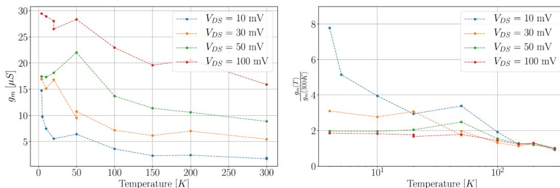
**Fig. 3.5.** Study of the transconductance enhancement effect in scaled FinFETs.
