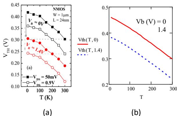
**Fig. 2.5** (a) experimental  $V_{TH}$  versus  $T$  at  $V_{DS} = 50\text{mV}$  and  $0.9\text{V}$ , and at  $V_B = 0\text{V}$  and  $1.4\text{V}$ . (b) modeled  $V_{th}$  vs  $T$  for  $V_d = 50\text{mV}$  and  $V_b = 0$  and  $1.4\text{V}$ .
