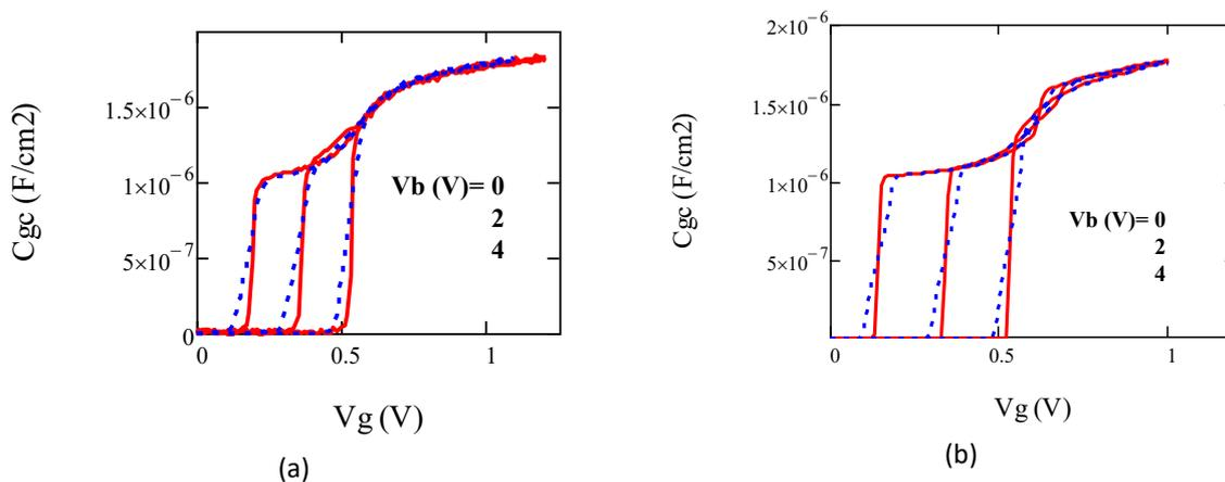
**Fig. 2.3.** Experimental (a) and modelled (b)  $C_{GC}(V_{GS})$  characteristics for NMOS GO1 devices ( $W=L=10\mu m$ ) at 4.2K for 2 AC levels: 40mV (red solid lines) and 1mV (blue dashed lines).
