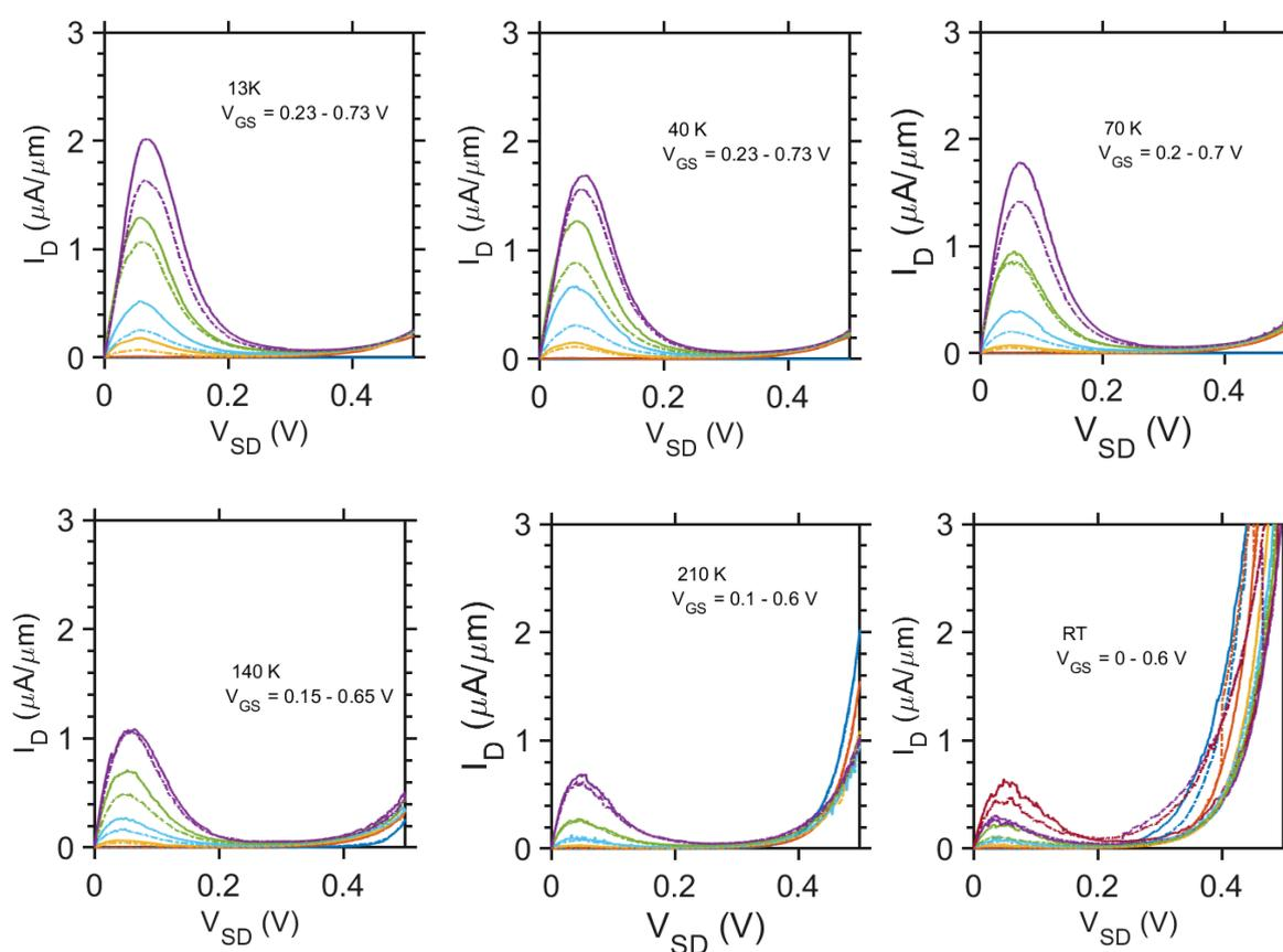
**Fig. 4.3:** NDR characteristics of a vertical nanowire TFET device with lower doping at different temperatures.
