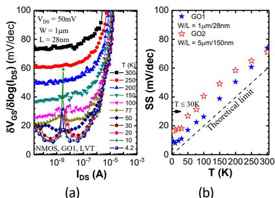
**Fig.2.7.** Extracted subthreshold current vs.  $I_D$  (a) and SS vs.  $T$  (b) for NMOS LVT, from 300K to 4.2K.
