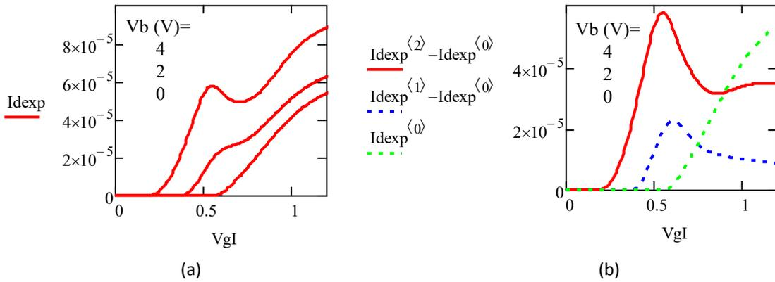
**Fig. 2.9.** a)  $I_d(V_g)$  characteristics at 4.2K for various  $V_b$  (0, 2, 4 V) and b) Back channel  $I_d(V_g)$  curves after subtraction of front channel component also shown in green dashed line.
