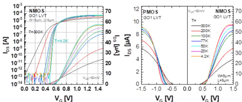
**Fig. 2.4.**  $I_d(V_g)$  characteristics for GO1 N and P MOS devices for various temperatures obtained in linear region ( $V_d=50mV$ ).
